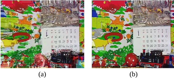
Fig. 3: Frame 75 of the “mobile and calender” sequence. QP=24, Average packet loss rate = 20%. Error Concealment using (a) “frame copy” algorithm, (b) “motion vector copy” algorithm.
